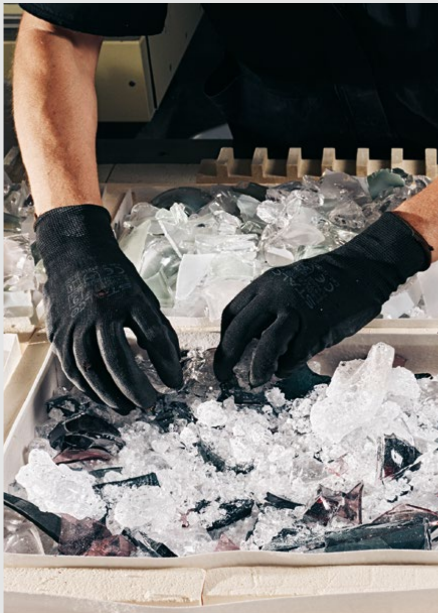
Each Fragmentglass panel is carefully assembled by stacking glass shards into a melting mold following DECHEMA Studio's precise recipe. The final result of each Fragmentglass plates carries an element of surprise as the melting process itself cannot be controlled.
