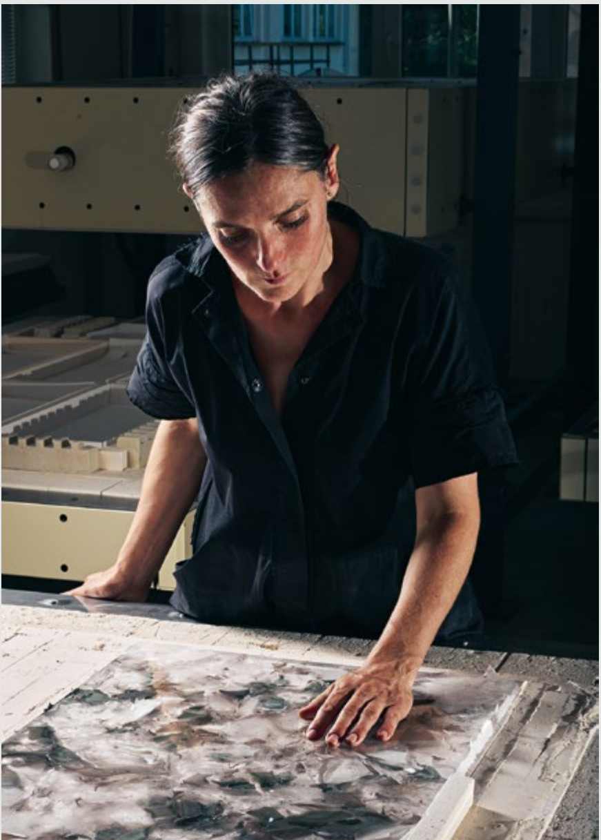
The development of individual colors for the panels was a complex and lengthy process. The designers continuously observed and evaluated how the pattern and structure of the shards arranged in the glass furnace appeared after melting. After many trials, Studio DECHEMA perfected three colors that can be beautifully combined in lighting designs or stand alone as visually strong elements.
