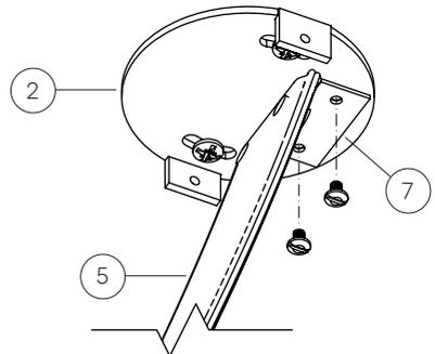
Slide the large and small canopy along the mounting to the ceiling and fix them to the anchor plates with a pair of screws.
